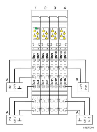
Figure 5 Typical connection of sensors
