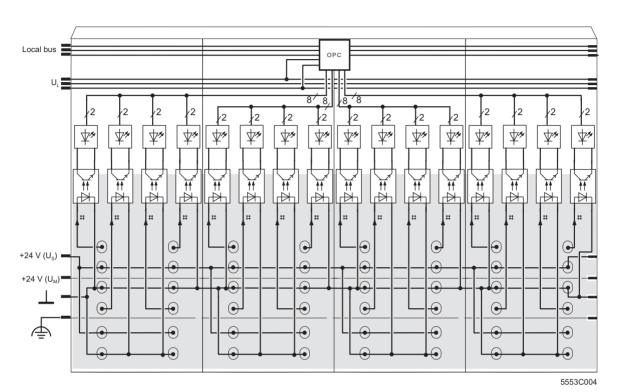
Figure 4 Internal wiring of the terminal points
